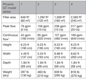
$<sup>^1</sup>$  Seccua always recommends a minimum 100  $\mu m$  fine filter to protect the membrane. Depending on the local water quality, an automatically rinsable 1-5  $\mu m$  pre-filter may be recommended. For free advice call +1 (503) 766 5551.
